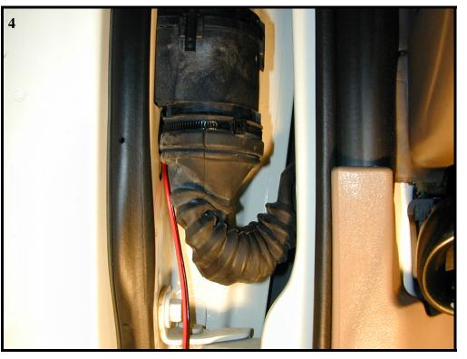
4. Pull the wire out between the door and door frame and remove any slack in the wire.
